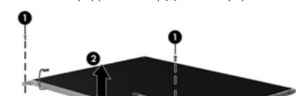
6. Remove the display panel assembly (2) from the display enclosure.
